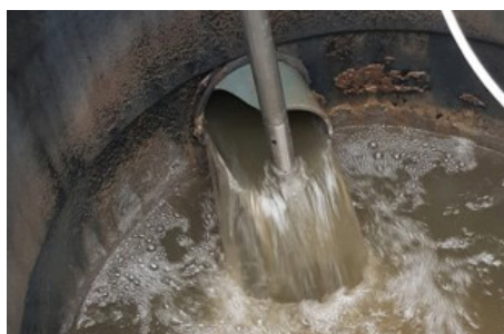
The SulfiLogger™ sensor placed directly in the raw sewage in the inlet of the well.
