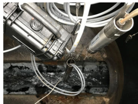
The SulfiLogger™ sensor measures H_2S directly in wastewater and in the air above.
