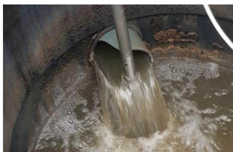
The SulfiLogger™ sensor placed directly in the raw sewage in the inlet of the well.
