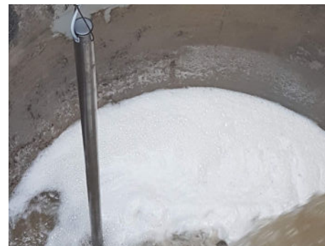
Figure 3: SulfiLogger™ H 2 S sensor with extension pipe in pump station sump.
